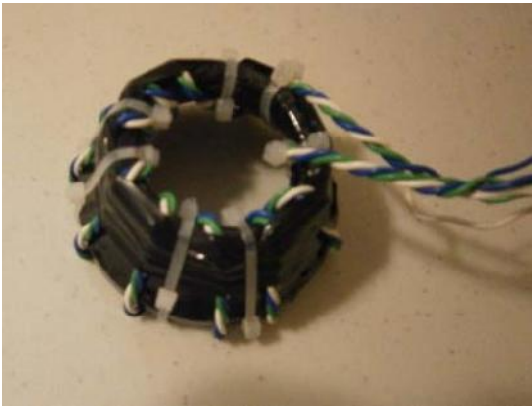
Figure 7 Unsymmetrical RF Transformer 1:9 on TV Yoke
