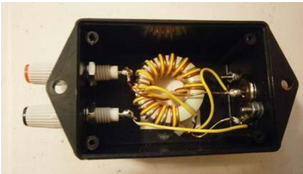
Figure 9 Unsymmetrical RF transformer 1:9 on the Base of Balun RBA- 1:1
