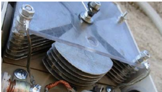
Figure 7 Capacitor of the UA6AGW Antenna V. 20-10.51
