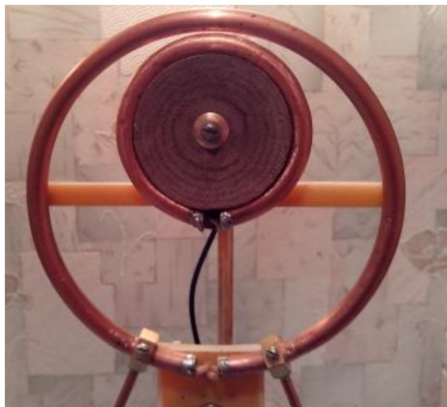
Figure 3 Coupling Loop at UA6AGW Antenna
