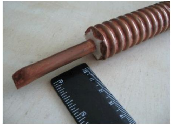
Figure 2 Coaxial cable "LCFS 114-50 JA, RFS (15239211)"
