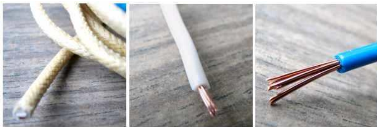
Photo 1 Examples of Some Good Antenna Strand Wires
