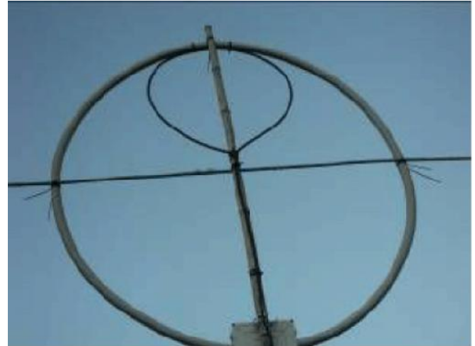
Figure 6 Coupling Loop on the Antenna Loop
