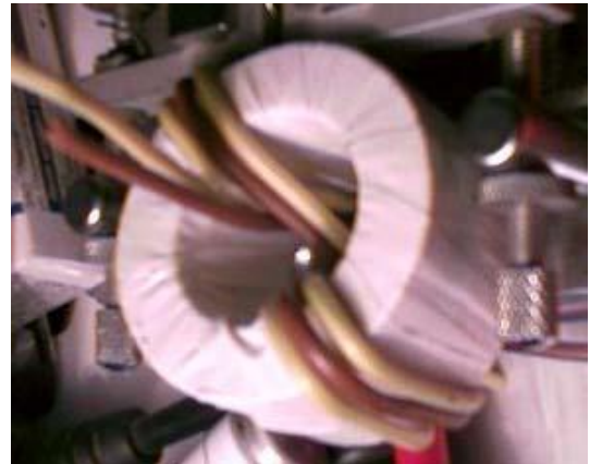
Figure 7 Ready Second Winding
