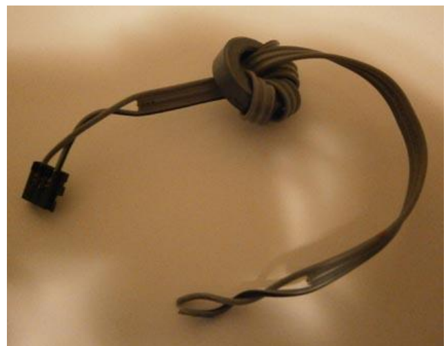
Cable with Ferrite Ring on it
