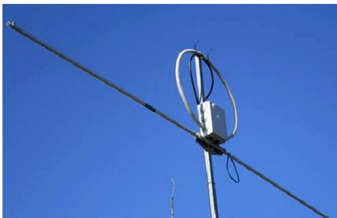
Figure 2 UA6AGW Antenna V. 20-10.51 on the mast
