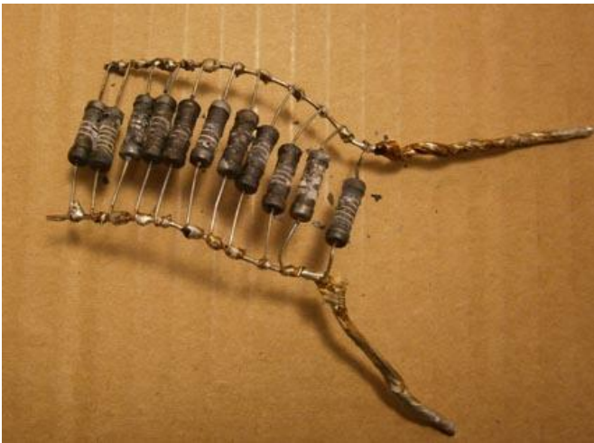
Burned Termination Resistor
