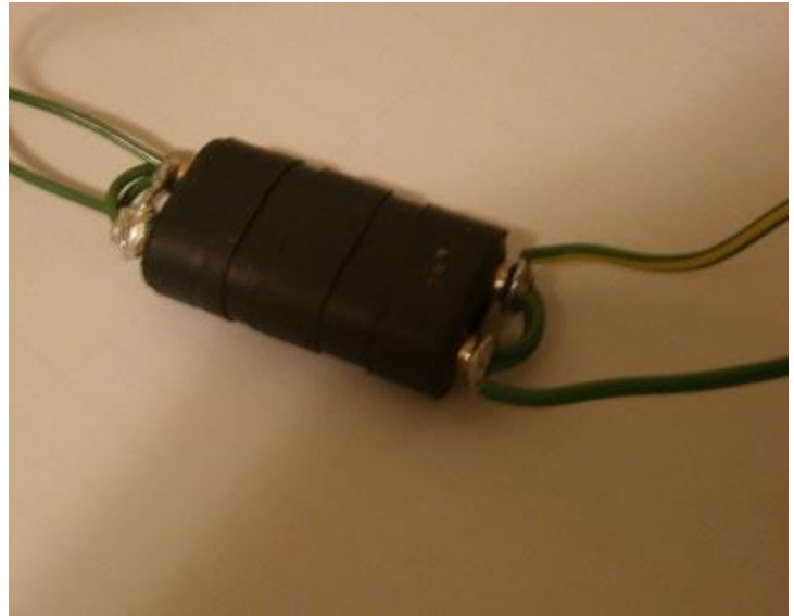
Ready Transformer with Insulated Windings
