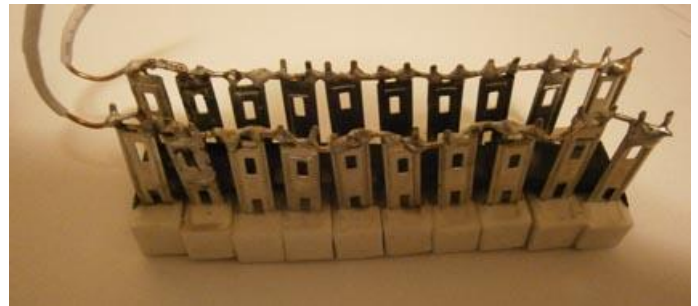
Termination Load on the Base of the Wire Wound Resistors
