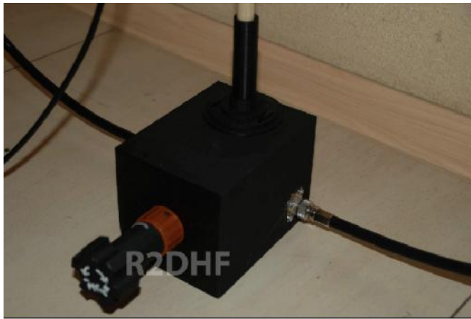
Figure 5 Plastic Box for Variable Capacitor
