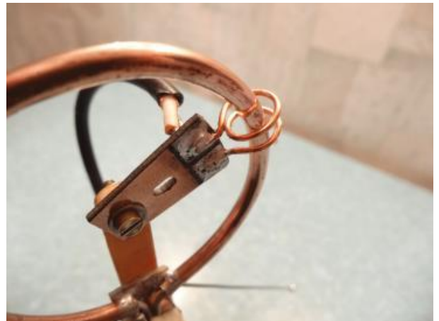
Figure 7 Fixture for Moving Coupling Loop
