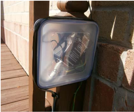
Figure 17 Transformer of Beverage Antenna in Closed Plastic Food Box
