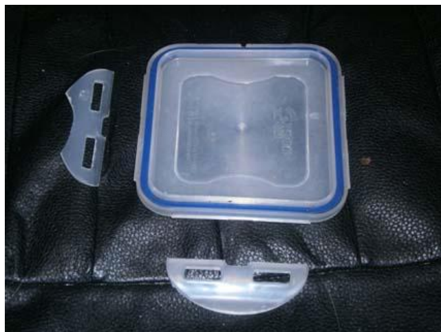
Picture 6 Cover with Cracked Retaining Tags
