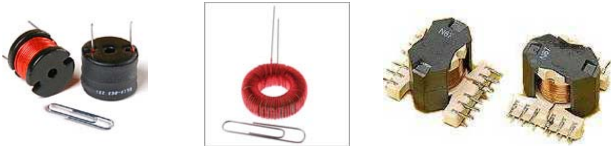
Coil Shapes ... Drum, Toroid & RM Style Coils and Cores (Wilco & Coilcraft)
