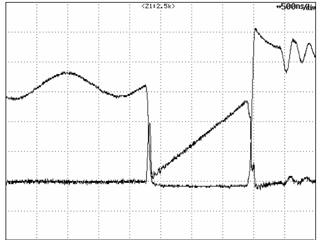
Figure 13 – 230 VAC, Full Load. Upper: I_{DRAIN} , 0.1 A / div. Lower: V_{DRAIN} , 100 V / div.
