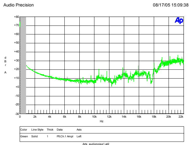
Figure 32 – Audible Noise V_{IN} = 230 VAC; I_{OUT} = 1.2 A.
