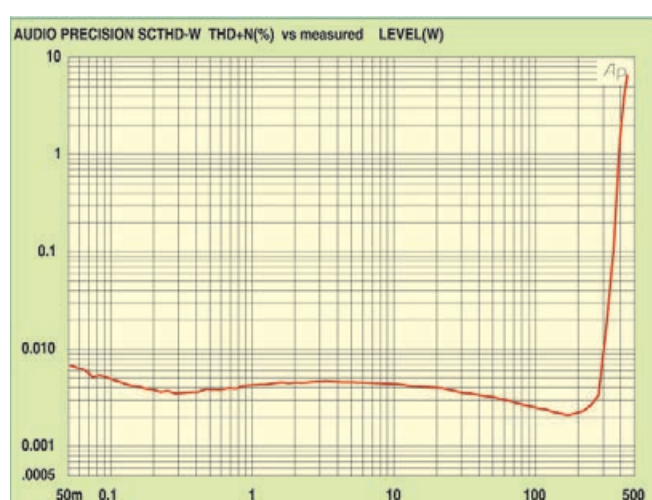
Fig.3: total harmonic distortion versus power at 1kHz into a 4-ohm load (10Hz-22kHz measurement bandwidth).
