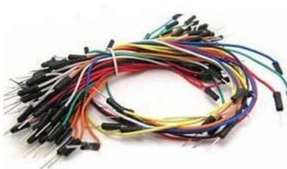
These are the 30 jumper leads that come with the breadboard
