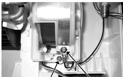
Screw of the motor band Screw of the ground wire
